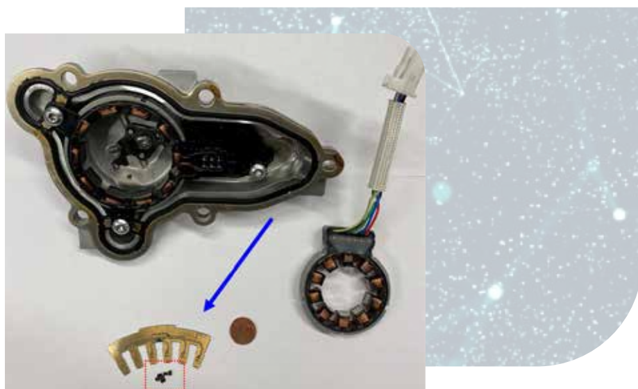
Figure 1. State-of-the-Art mechanical BEV resolver is replaced by integrated sensor array
