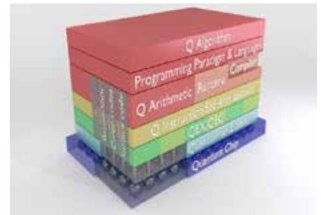
Fig. 4: Overall system stack embedding quantum algorithms, compilers (red) at room temperature; quantum control (yellow and green), and quantum classical interfaces (light blue) at intermediate 1-10K temperature levels; to the qubits (blue) at mK temperature.
